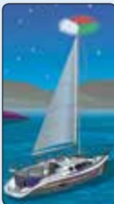
*An alternative to the sidelights and sternlight is a combination red, green, and white light, which must be exhibited near the top of the mast.*
