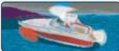
*The masthead light and sternlight may be combined as an all-round white light on vessels less than 39.4 feet long.*
